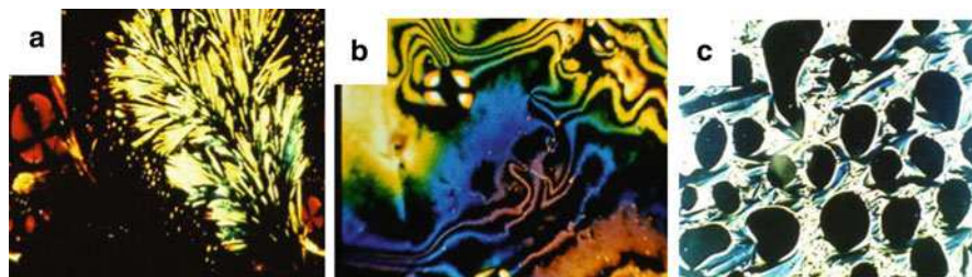
Fig. 1.3 Photo-image of a 20 \mu\text{m} thick polycrystalline layer of cholesteryl acetate placed between two cover glasses in crystalline phase (a), cholesteric phase (b) and at the transition from the cholesteric to isotropic phase (c)
